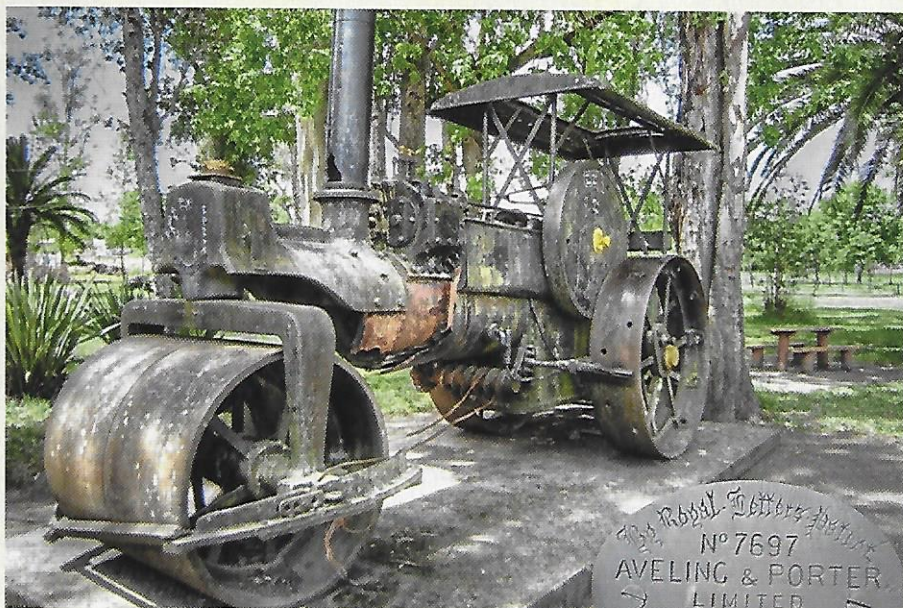
The roller in the park with, inset, its Royalty plate. Note the interesting and somewhat non-standard injector clack and the spike holes in the original [and somewhat thin - by now] rolls. The awning has been modified over time as well. Photos: J M Techera, courtesy of Miguel Montelongo
